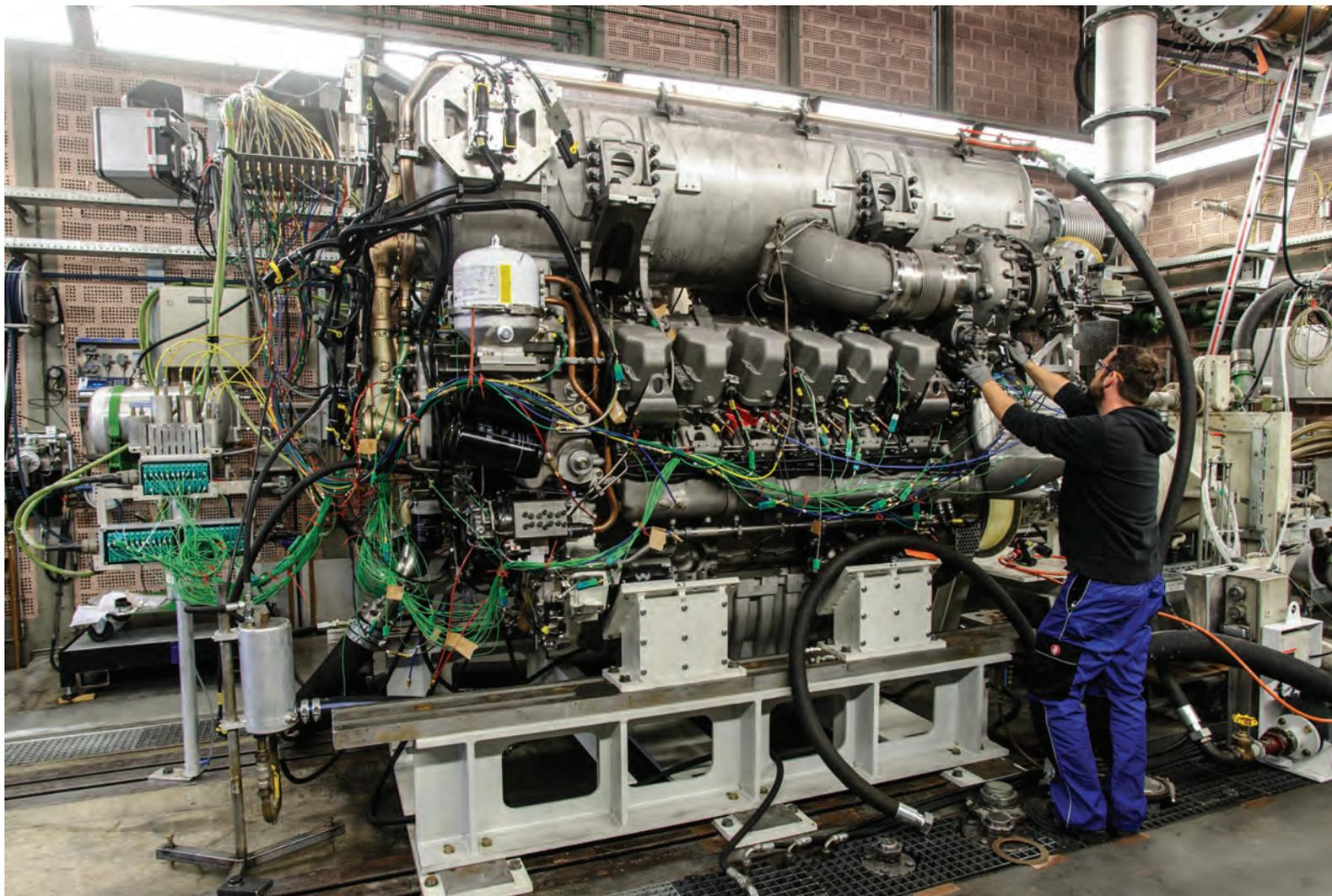
Figure 1 – MTU 12V4000U83 Submarine Diesel under Test
